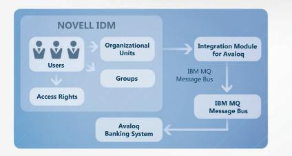
The Integration Module uses the the IBM MQ message bus architecture for the data exchange. This way the solution integrates seamless in your existing SOA architecture. By default the modul is configured as a one way communication interface and exclusively sends information to Avalog.
