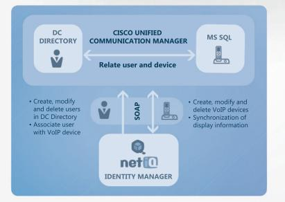
Our integration module uses the AXL SOAP interface for the synchronization with the CUCM. The AXL SOAP server is an integrated part of the CUCM solution. It provides a very flexible and customizable interface for the data exchange.
