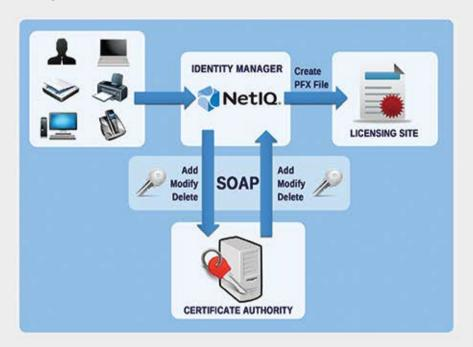
Based on the Open Source Certificate Authority (CA) EJBCA (www.ejbca.org) the integration module automatically creates certificates for any objects (such as users, servers, workstations, laptops, printers, telephones, etc.) in the central directory. EJBCA is a CA based on JEE technology and can be used as a complete PKI infrastructure for large companies.
